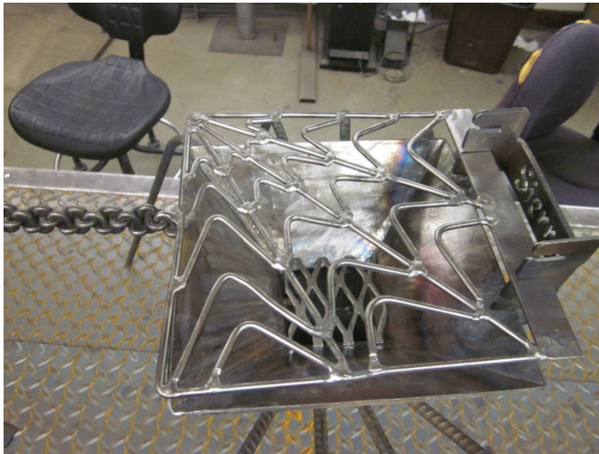
Worksheet #7 infused math into the design and construction of the grill. Students were then allowed to design and fabricate a custom grill, calculating the total length of 3/16" rod and the total cost of materials as part of their final project.
